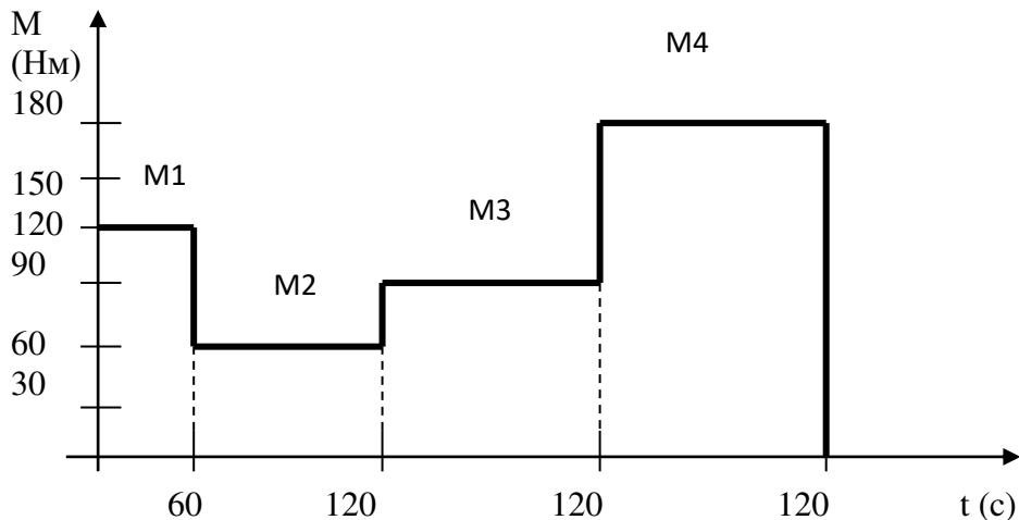
$$\begin{aligned} 2. \text{ Находим } M_{\text{э}} &= \sqrt{\frac{M_1^2 t_1 + M_2^2 t_2 + \dots + M_n^2 t_n}{t_1 + t_2 + \dots + t_n}} = \\ &= \sqrt{\frac{120^2 \cdot 60 + 60^2 \cdot 120 + 80^2 \cdot 120 + 170^2 \cdot 120}{60 + 120 + 120 + 120}} = 110 \text{ (Нм)} \end{aligned}$$
