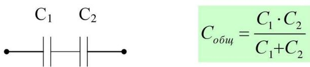
$$C_{общ} = \frac{C_1 \cdot C_2}{C_1 + C_2}$$
