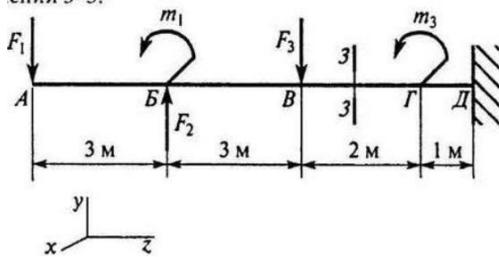
$F_1 = 10 \text{ кН}; F_2 = 20 \text{ кН}; F_3 = 28 \text{ кН};$
